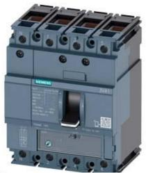
CIRCUIT BREAKER 3VA1 IEC FRAME 160 BREAKING CAPACITY CLASS S ICU=36KA @ 415 V 4-POLE, LINE PROTECTION TM220, ATFM, IN=25A OVERLOAD PROTECTION IR=17,5A ...25A SHORT CIRCUIT PROTECTION II=12,8 X IN NEUTRAL UNPROTECTED CABLE CONNECTION
